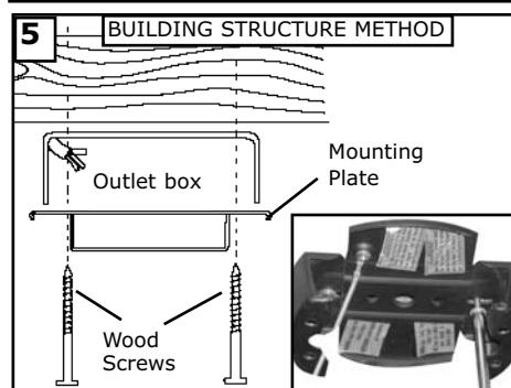
Secure mounting plate directly to a joist from the building structure via the two knock out holes on the outlet box. Use only the appropriate wood screws and washers included with your fan. Caution: Wood screws must go through into the building joist.
